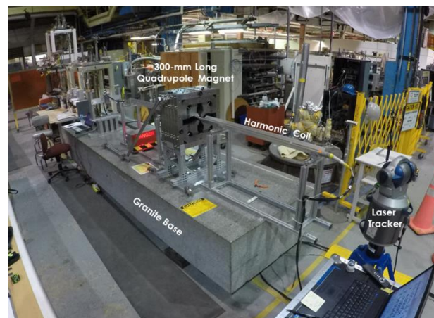
Fig. 5. Field harmonics test setup with harmonic coil and laser tracker mounted on the granite base.
